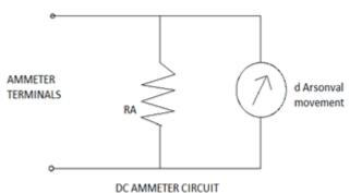
1 mA flowing through coil implies that 9mA must be diverted through RA. V = ir20 \* 10<sup>-3</sup> = 9 \* 10<sup>-3</sup> R<sub>A</sub>
